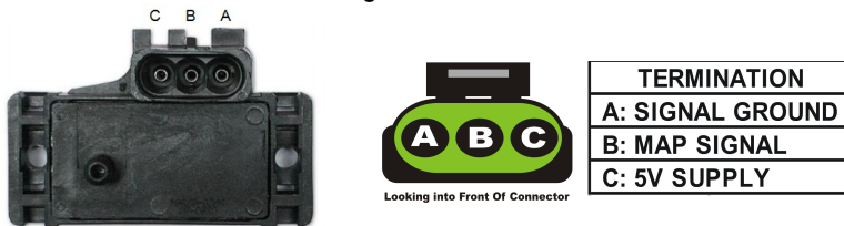
Figure 5 – Manifold Absolute Pressure Sensor and harness Termination
