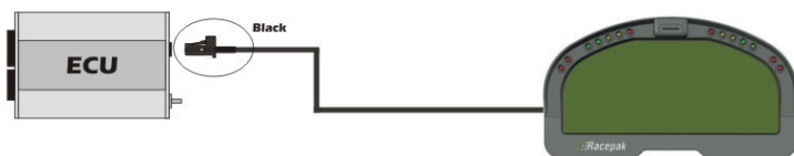
Figure 12 – Haltech ECU connected to a Racepak Dash
