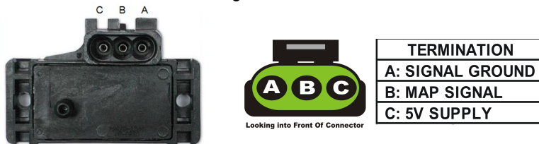
Figure 5 – Manifold Absolute Pressure Sensor and harness Termination
