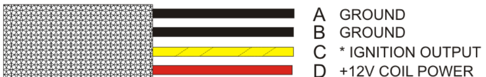
Figure 10 – Haltech Flyloom Ignition Harness Connections
