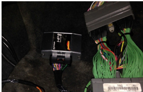
Figure 4 - Haltech HPI and Harness Connected
