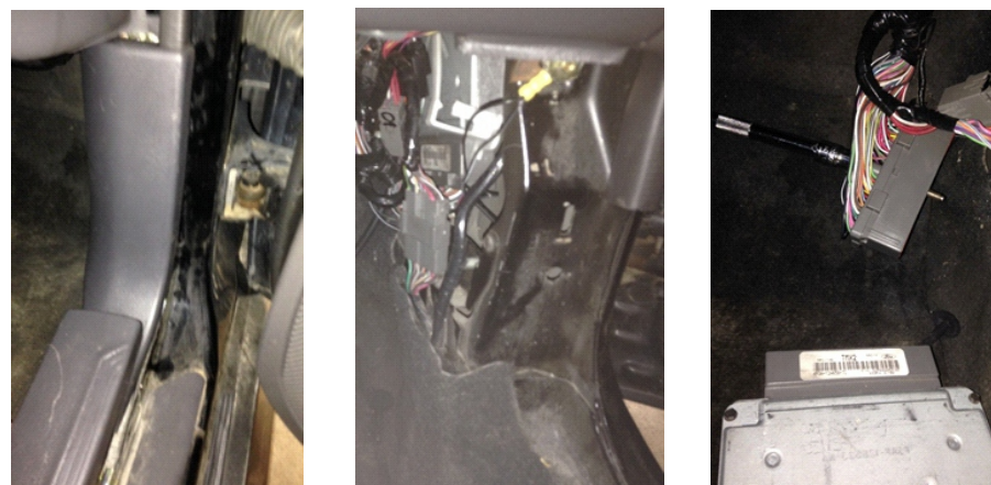
Figure 2 - Factory ECU Location
