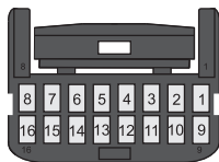
AUXILIARY CONNECTOR (16 PIN) REAR VIEW (WIRE SIDE)
