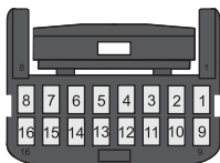
AUXILIARY CONNECTOR (16 PIN) REAR VIEW (WIRE SIDE)
