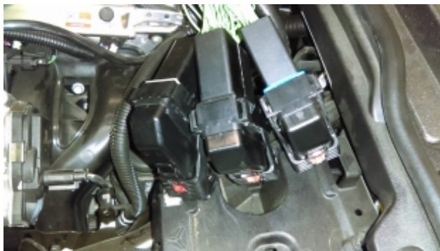
Figure 2 - Connecting Haltech Harness to Factory Harness
