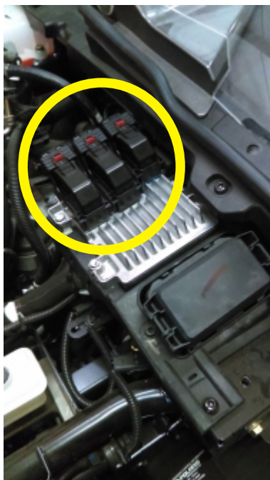
Figure 1 - Factory ECU Located in the Engine Bay
