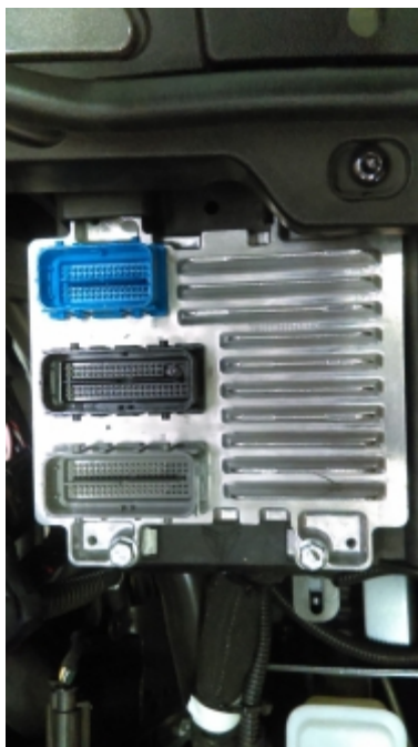
Figure 1 - Factory ECU Located in the Engine Bay
