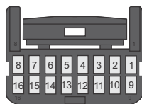
AUXILIARY CONNECTOR (16 PIN) REAR VIEW (WIRE SIDE)
