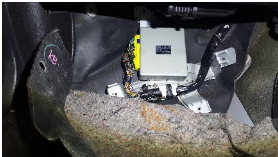
Figure 3 - Factory ECU is now ready for removal.
