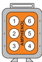
CAS BREAKOUT SIDE CONNECTOR PINOUT HARNESS SIDE VIEW
