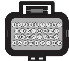
iC-7 Main connector (AMP 34-pin Keyway 2) Wire side view
