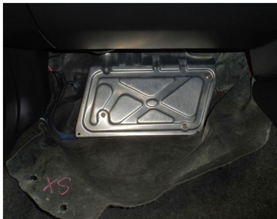
Figure 2 – ECU Protection panel under the carpet
