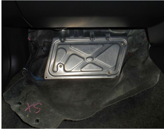
Figure 5 – ECU Protection panel re-installed
