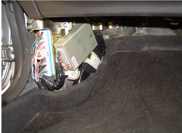
Figure 4 – Haltech ECU Installed
