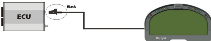
Figure 9 – Haltech ECU connected to a Racepak Dash
