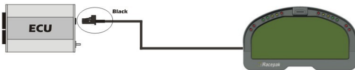
Figure 9 – Haltech ECU connected to a Racepak Dash
