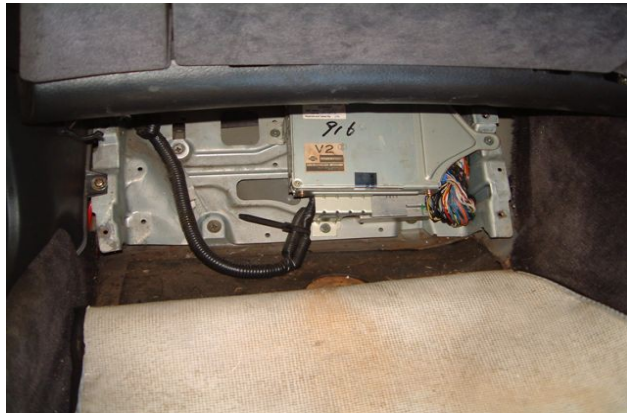
Figure 2 – Factory ECU Mounting Location with cover removed
