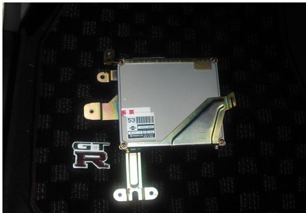
Figure 2 – Factory ECU disconnected and removed
