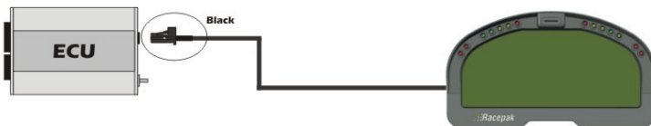
Figure 8 – Haltech ECU connected to a Racepak Dash
