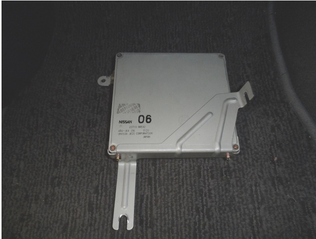
Figure 2 – Factory ECU disconnected and removed
