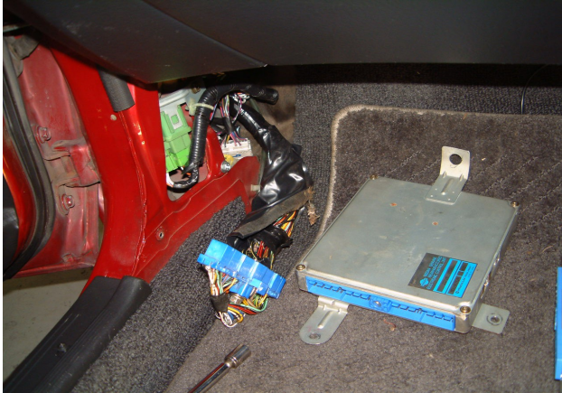
Figure 2 – Factory ECU disconnected and removed
