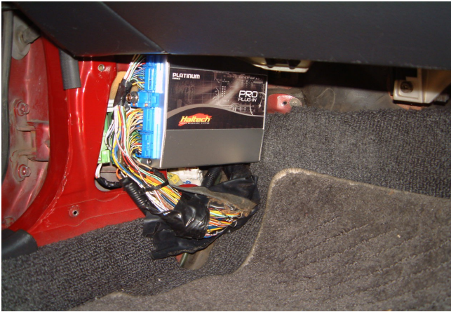
Figure 6 – Platinum Pro Plugin Mounted in a R32 GTR.
