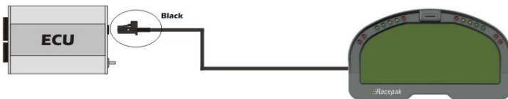
Figure 9 – Haltech ECU connected to a Racepak Dash
