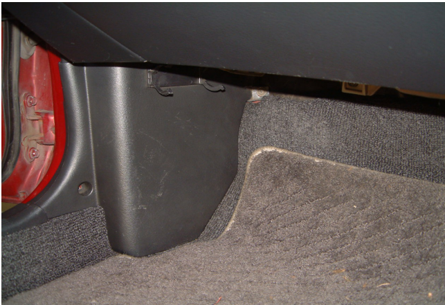
Figure 7 – Kick panel Re-installed
