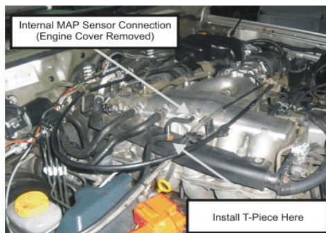
Figure 6 Internal MAP Sensor Connection to Engine Manifold (Engine Cover Removed)
