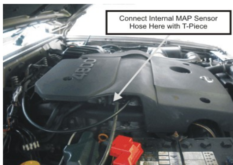
Figure 5 Internal MAP Sensor Connection to Engine Manifold
