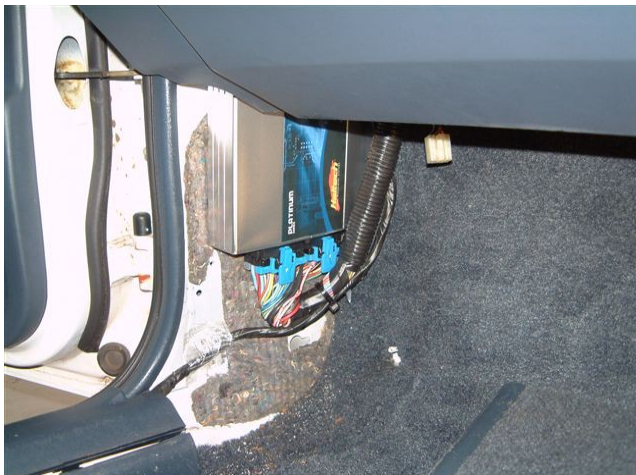
Figure 3 – Haltech Sport GM Mounted in vehicle
