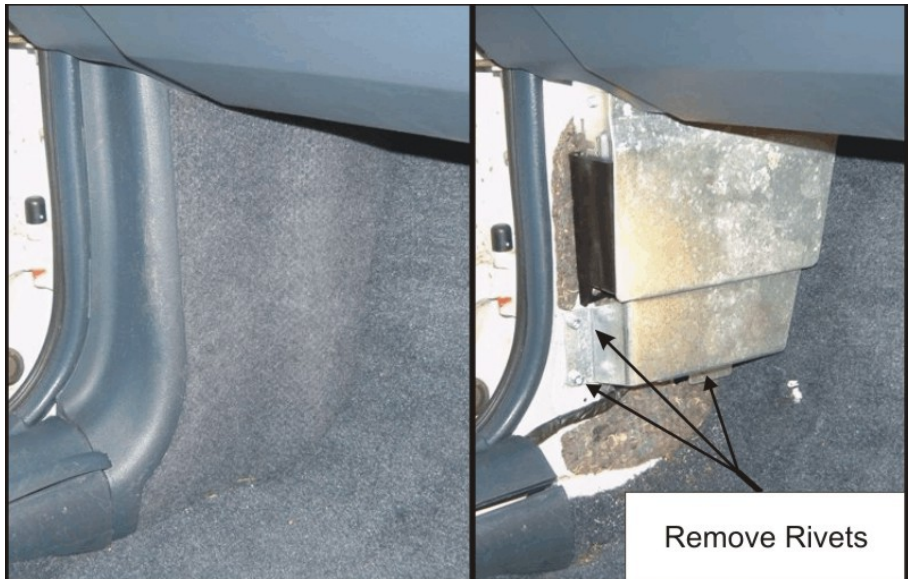
Figure 1 – ECU Location with security cover installed
