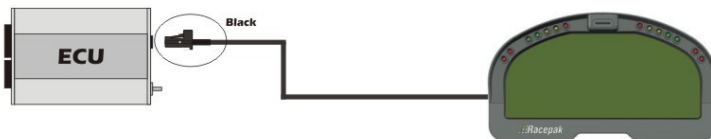
Figure 7 – Haltech ECU connected to a Racepak Dash
