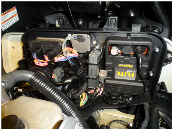
Figure 7 – Location of WBC1 on PWC Installation
