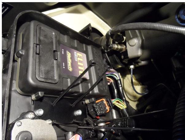
Figure 3 – Elite ECU Mounted
