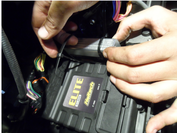
Figure 6 – Securing the WBC1 to the Elite Mounting Bracket
