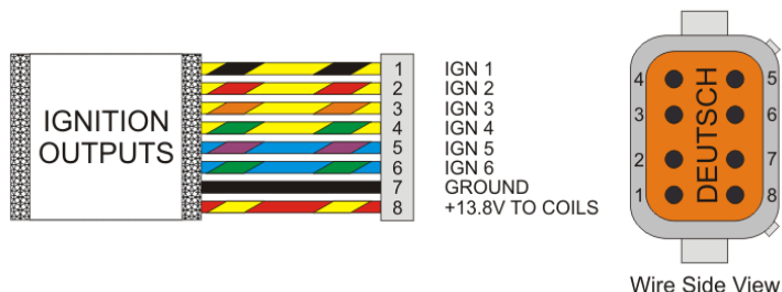
Figure 1 – Ignition Breakout Connector wiring
