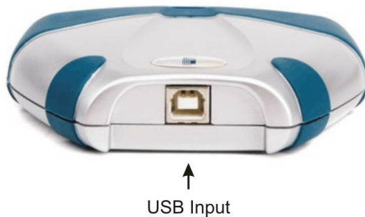
Figure 2- Haltech Stingray 2 Channel USB Oscilloscope rear panel connection
